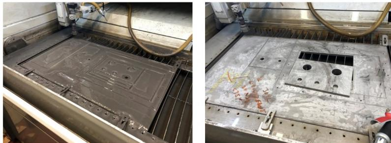
FIGURE 3.12: Photographs of water-jet cut SS304 plates. The right picture was taken after flushing from the surface of the plates the water/abrasive mixture sprayed out from the jet cutter.
